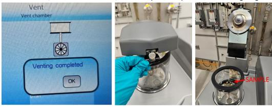
5. Close the lid, and run **Timed Au/Pd** recipe. It is not recommended to skip the "Outgas Chamber" step, that is part of the recipe. The deposition process is set for 15 sec, that would deposit about 5 nm Au/Pd. After 15 sec, the plasma turns off, and the chamber starts venting.
